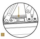
To gain access to the outside of the window for cleaning, open window to the stop position and then close slightly. Press the buttons (Fig 3) on top and bottom of window.
