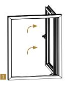
If a safety restrictor in not fitted, the fire escape position is achieved by fully opening the window to 90 degrees (Fig 1).
