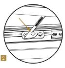
2 If a safety restrictor is fitted, open the window to the stop position and then close slightly. Release the arm from the stud (Fig 2) for window to fully open. The restrictor will self relocate when window is closed.
